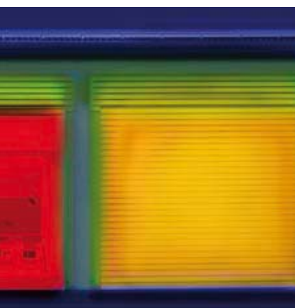
This thermal image of a conventional sectional door clearly shows the loss of heat to the outside.
